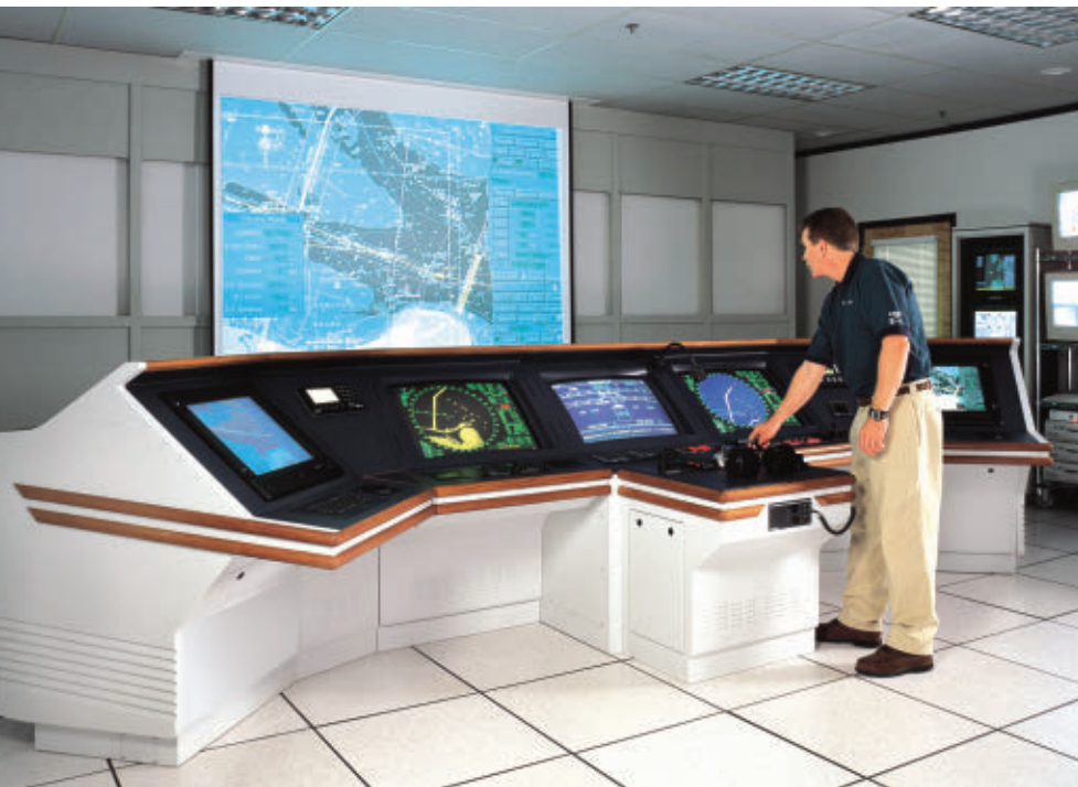
The Northrop Grumman Sperry Marine Voyage Management System training center in Charlottesville, Va., blends several kinds of navigational sensors for enhanced shipboard navigation.
